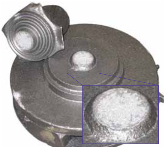
Figure 6 Sectioned casting after shakeout showing feeder contact after knock off
