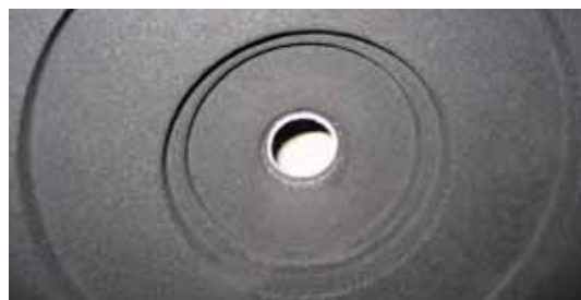
Figure 5 Cope pattern layout and cope casting cavity
