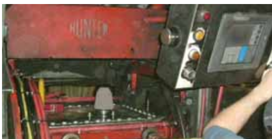
Figure 3 Casting layout and sleeve on pattern plate
