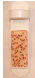
Figure 2 Dip slide showing bacterial growth due to contaminated water source
