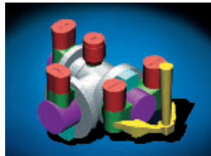
In-line gating system with two no. 6 prints
