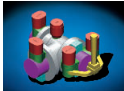
In-line gating system with STELEX filter print 7
