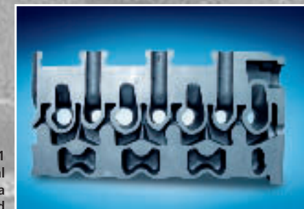
Figure 1 Complex internal passages of a cylinder head
