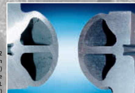
Figure 2 Veining defects in turbo housing (left) eliminated by the use of RHEOTEC XL (right)
