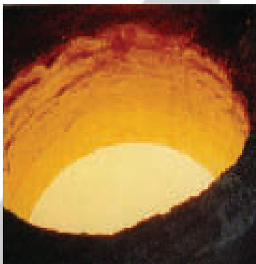
The furnace is ready for the second tap. NOTE the CLEAN METAL and LINING SURFACE.
