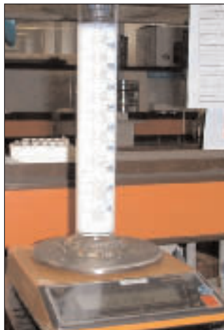
Figure 11 - Density measured by weight and volume
